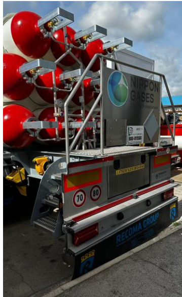
Hydrogen high flowrate tube trailer
